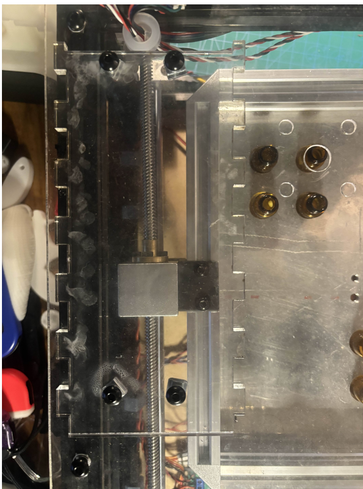
Figure 50: Syringe motor mounted onto top acrylic panel with sealed wire pass-through.
