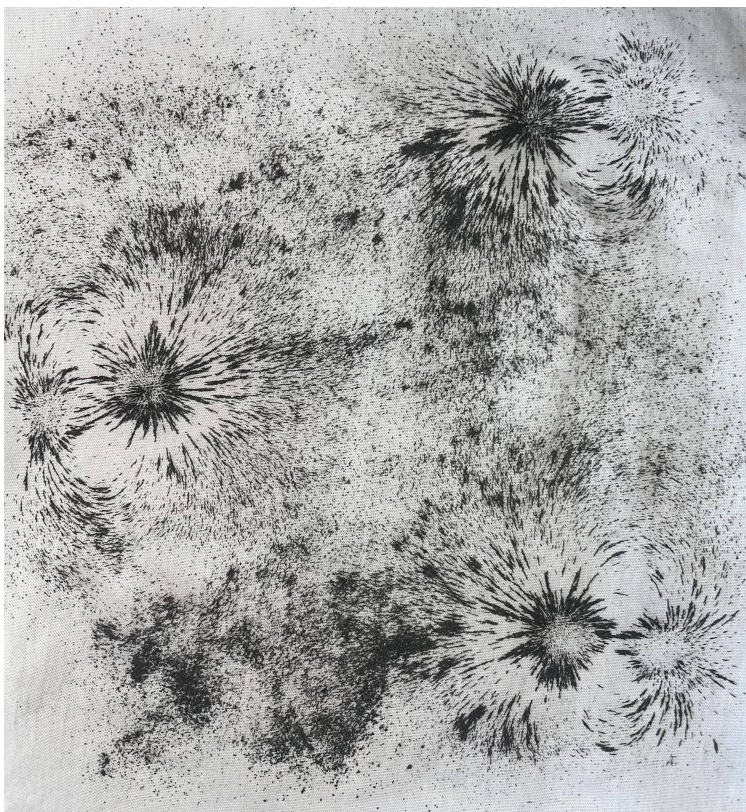
Figure 16: Magnetic field interference test using magnetic sand. The distinct, non-overlapping patterns confirm that each mixing motor generates an isolated magnetic field, preventing interference between adjacent vials.
