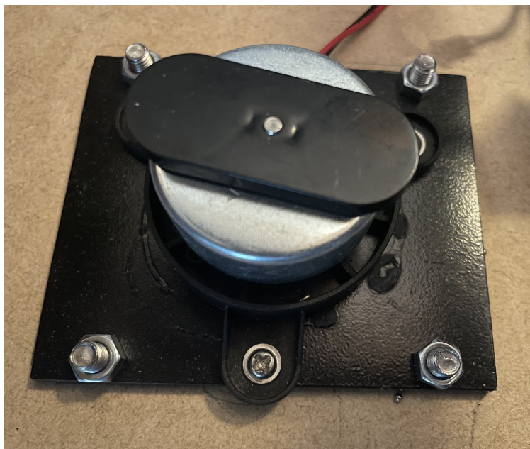
Figure 13: 12V DC motor with large magnet attached for magnetic agitation.
