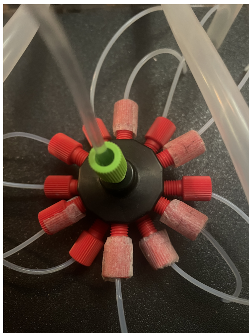
Figure 9: Manifold used to split flow from syringe pump into the 12 vials
