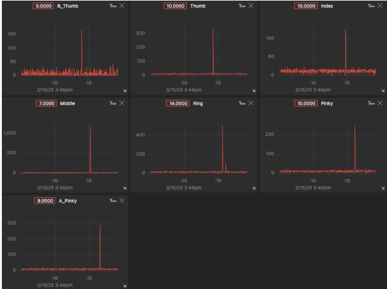
Image(7): Peak voltage output of Piezoelectric sensors for each finger
