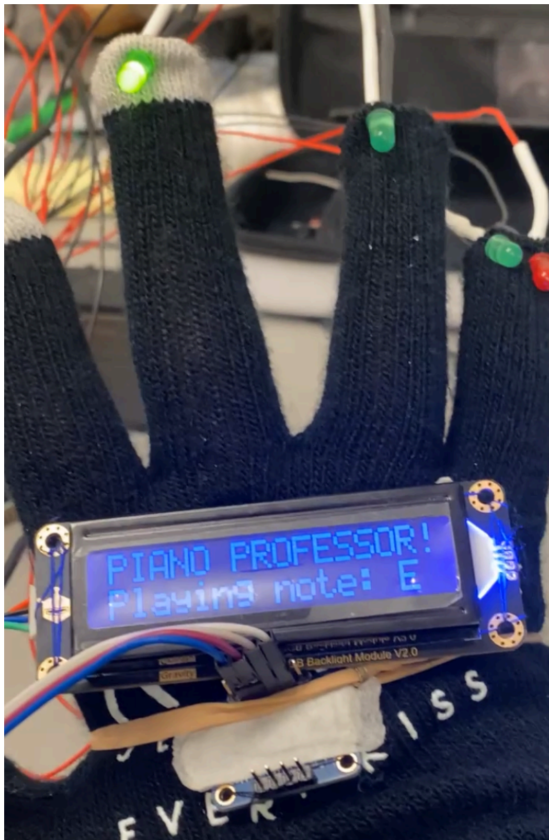
Image(9): LCD Display in Freeplay with Previous Note's LED
